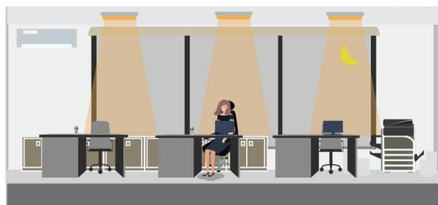
When ambient light is not sufficient, the sensor detects a moving object and the light comes on automatically.
