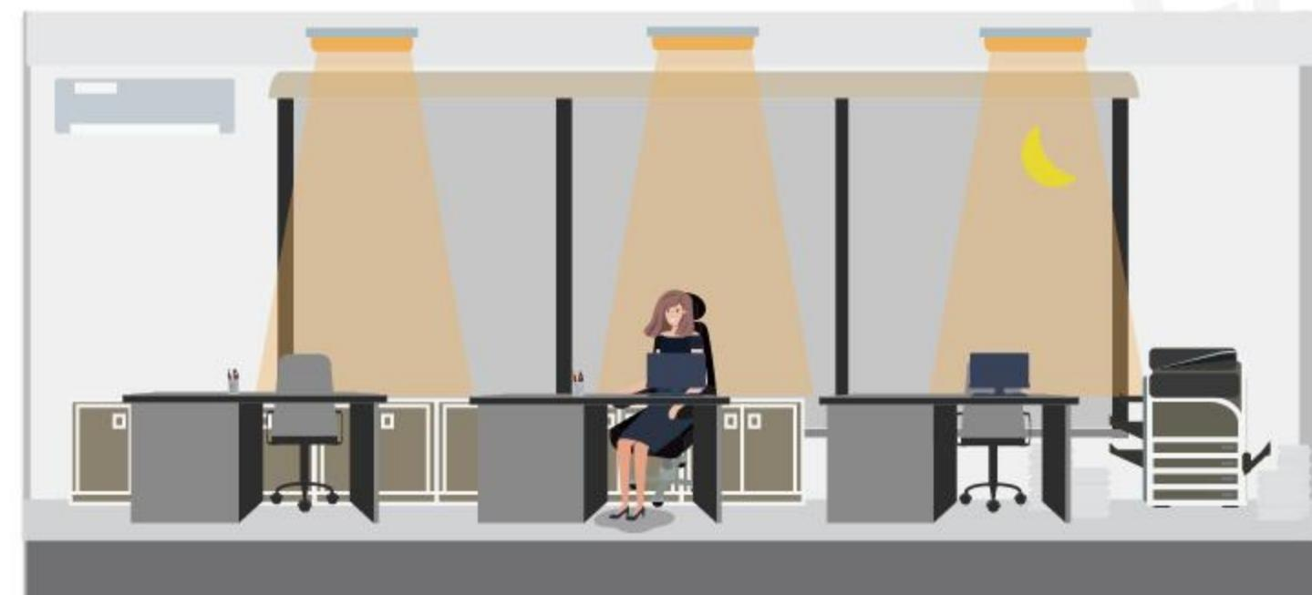
When the ambient light is insufficient, the sensor detects moving objects and the light automatically lights up
