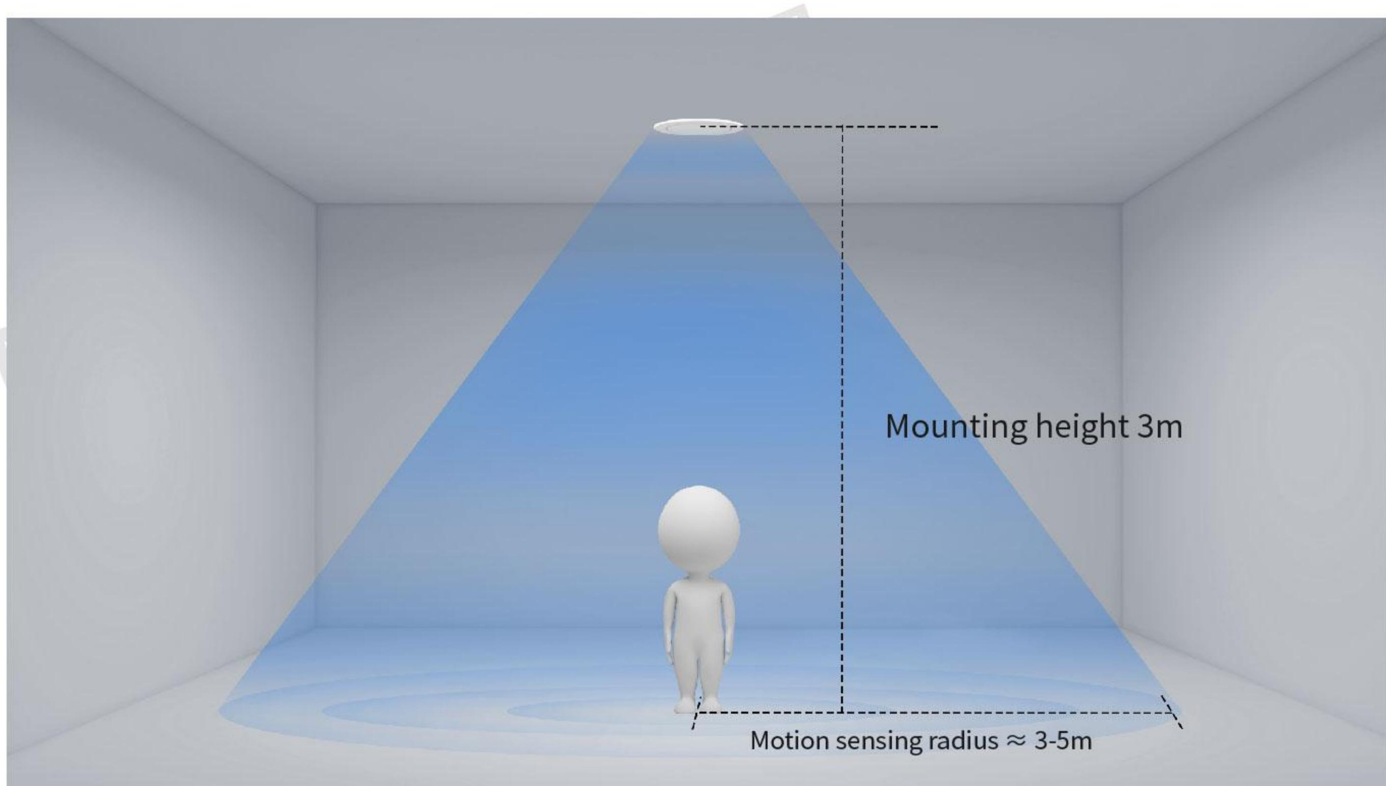
Radar Sensing Schematic
