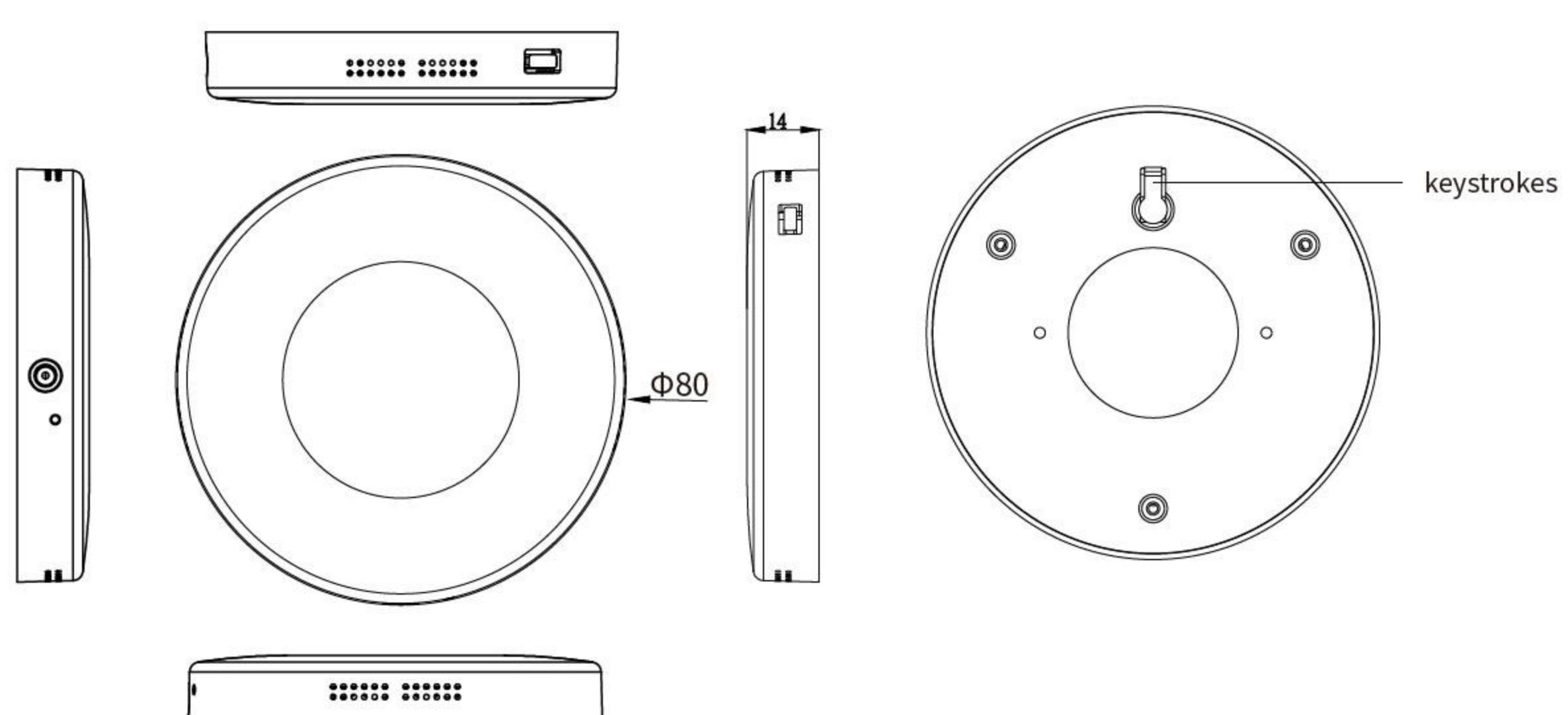
The finished product has a DC power interface bit, and the network button, reserved RS232 serial port. When you want to connect to the network, first press it twice quickly and then press it for more than 1 second after releasing it, then release it to enter the network mode. Serial port holder pin counterclockwise order are 5V, Tx, Rx, GND (when using the reserved serial port, please open the block first).
