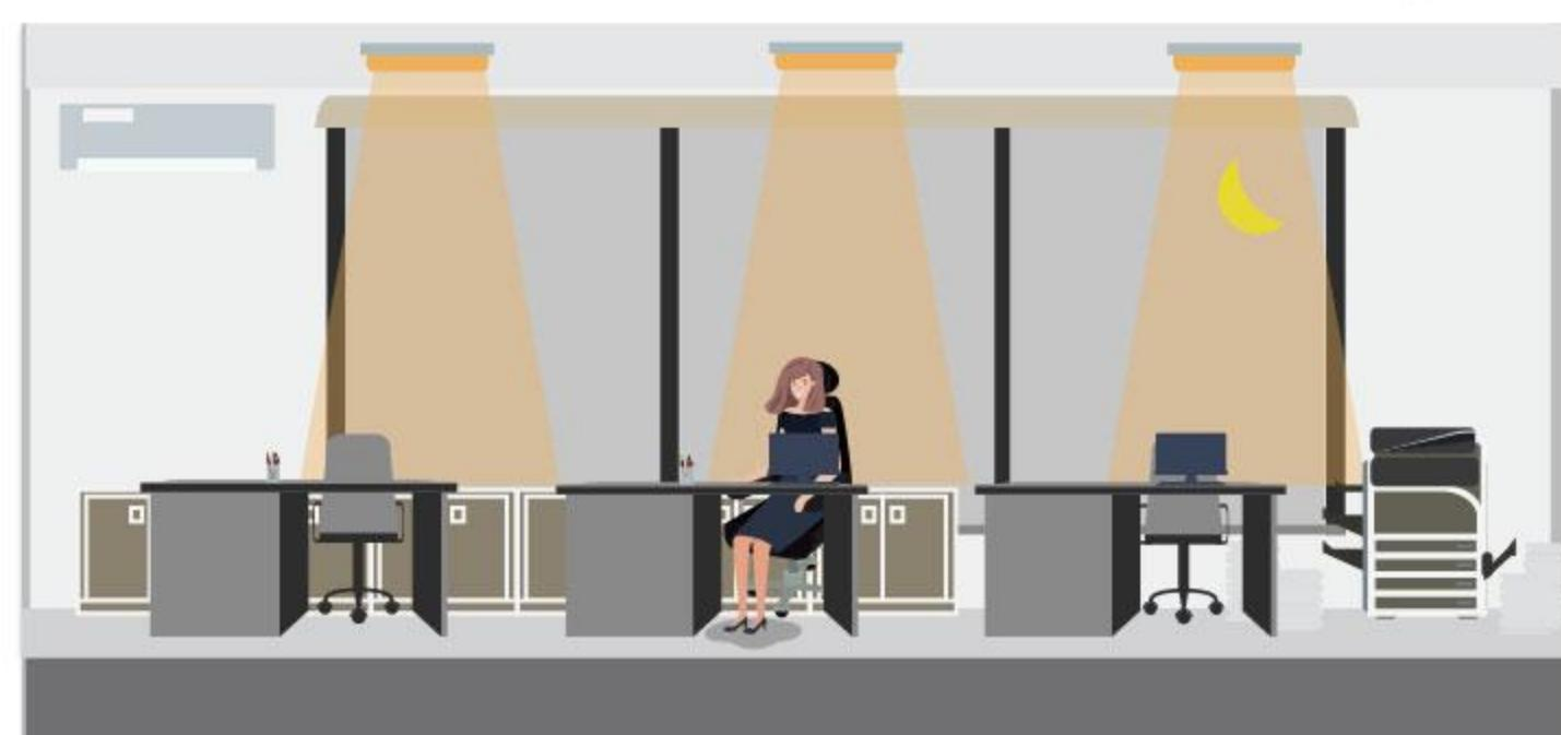
When the ambient light is not sufficient, the sensor detects a moving object and the light comes on automatically.
