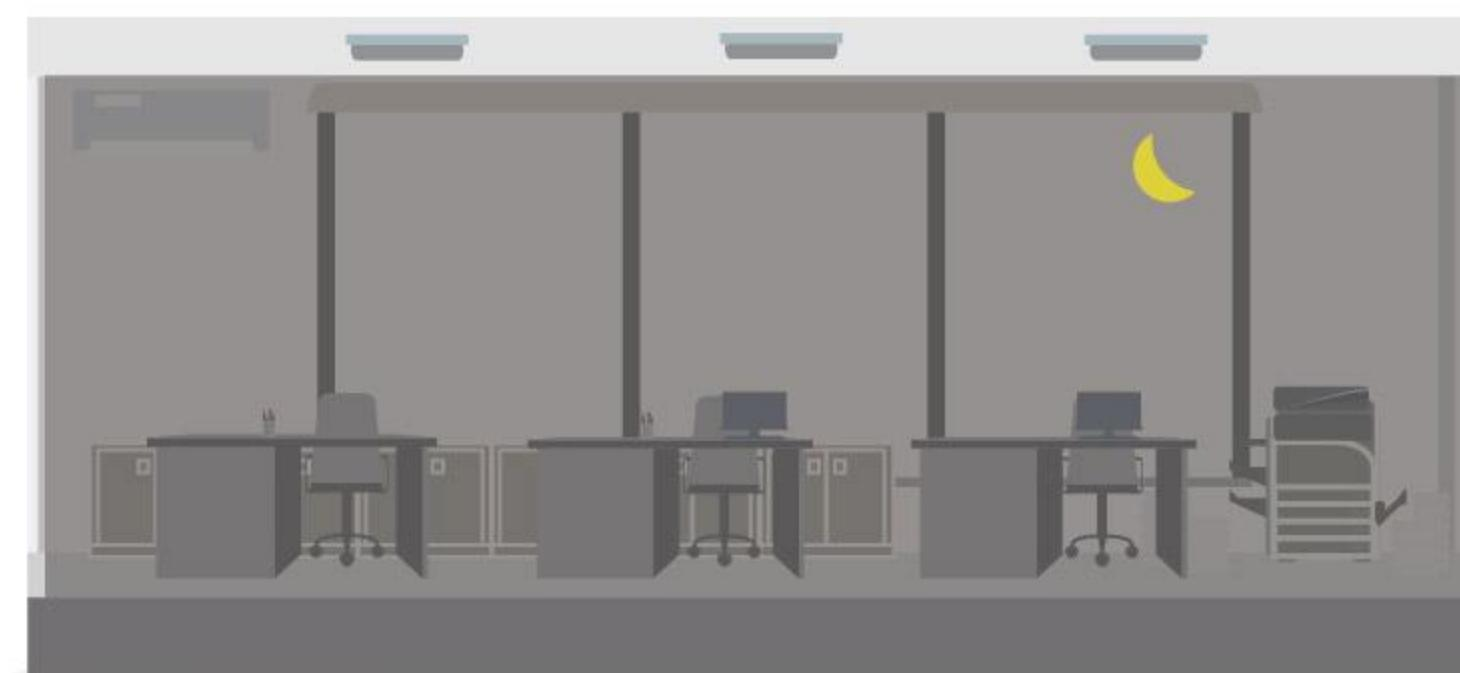
The moving object leaves. After the preset delay time has elapsed, the light goes out automatically.
