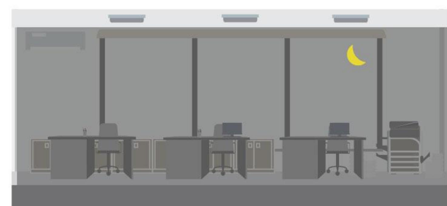
The light goes out automatically after the preset delay time has elapsed when the moving object leaves.
